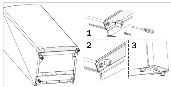
Tilt the appliance slightly back and block it in this position. Use the delivered screw to secure the
